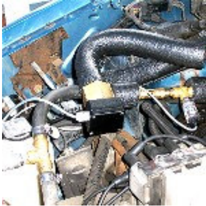
Figure 2 Photograph of the Series 600 refractive index sensor installed in the liquid line of a 1994 Dodge Caravan air conditioning system.
